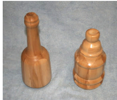
Frank Calzaretta - A mallet and box. Both are made from maple bowling pins. Finished with Myland friction high build.
