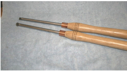
Gene Combs - Two turning tools made from ash, and finished with lacquer.
