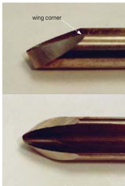
The side profile of Lyle Jamieson's favorite grind has nearly a straight line from the tip to the wing corner.
