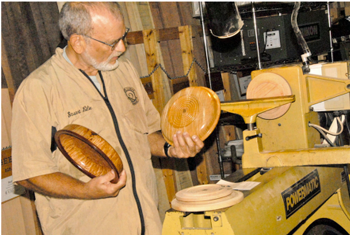
Stuart Lillie demonstrated how to finish platters and bowls using the mortise and how to put rings on the bottom.
