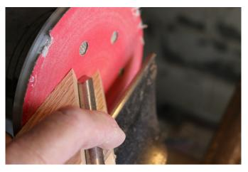
a sanding disk to grind the wing angle.
