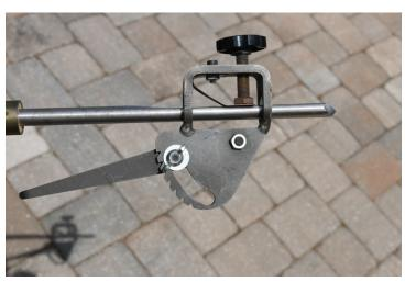
Begin sharpening by grinding the wings first, here is the right wing when I started to sharpen it. Notice the flat at the cutting edge.
