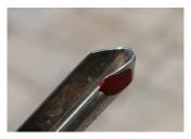
Continue sharpening the right wing until there is no reflection from the cutting edge and then go on to sharpen the left wing. Once both wings are sharpened blend
